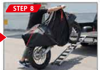
Wrap a tie-down soft hooks around the handlebar then load onto a truck.
