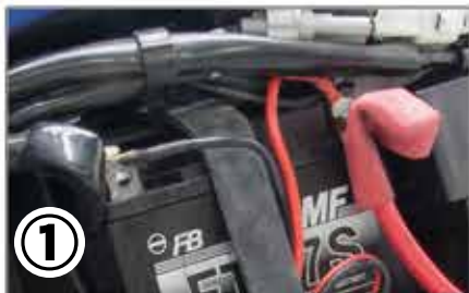
Install the battery charging harness to your bike.
