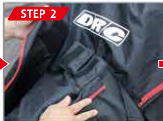
Lace the velcro flap into the loop on the front fender and secure.
